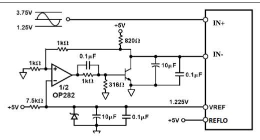
Figure 7-20. External Reference and Low Impedance Buffer
