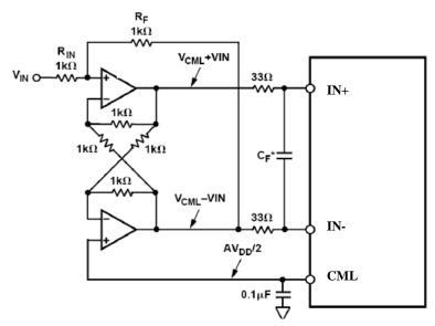
Figure 7-9. Cross-Coupled Differential Driver
