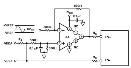
Figure 7-12. Single-Ended Input with DC-Coupled Level Shift
