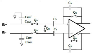
Figure 7-3. B9240MGRH Simplified Input Circuit
