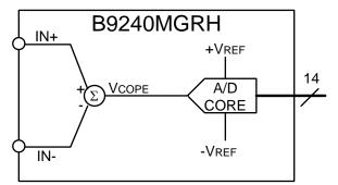
Figure 7-2. B9240MGRH Equivalent Functional Input Circuit
