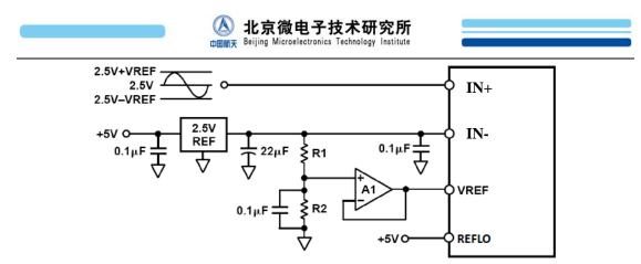
Figure 7-18. External Reference,  $V_{CM}$  = 2.5 V (2.5 V on IN-, Resistor Divider to Make  $V_{REF}$ )
