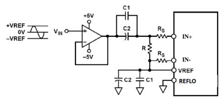
Figure 7-13. AC-Coupled Input
