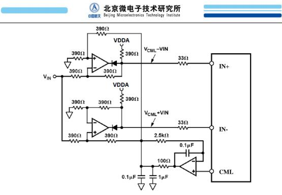
Figure 7-10. Differential Driver with Level-Shifting
