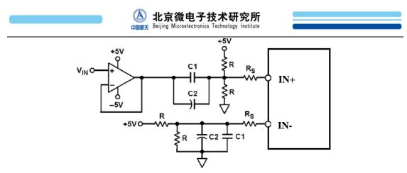
Figure 7-14. AC-Coupled Input-Flexible Input Span, V<sub>CM</sub> = 2.5 V
