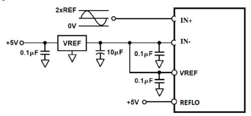
Figure 7-19. Input Range = 0V to  $2 \times V_{REF}$
