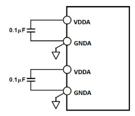
Figure 7-23. Analog Supply Decoupling
