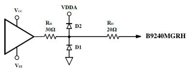
Figure 7-7. Sample Clamping Circuit
