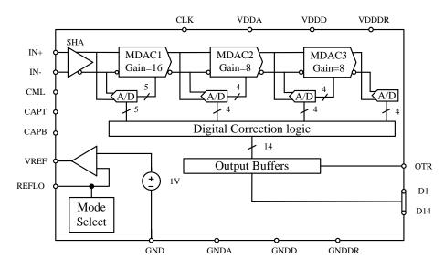
Figure 3-1. Functional Block Diagram
