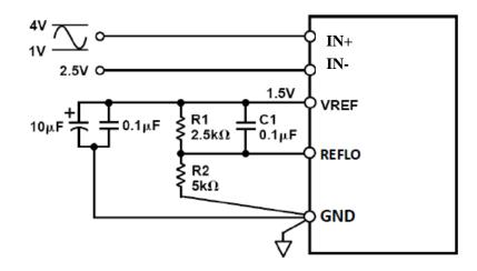
Figure 7-17. Resistor Programmable Reference (3V p-p Input Span, V<sub>CM</sub> = 2.5V) 7.10 Using an External Reference
