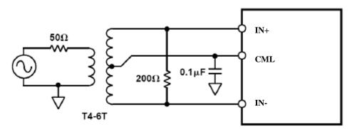
**Figure 7-8. Transformer Coupled Input**
