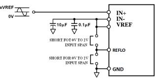
Figure 7-15. Internal Reference (2V p-p Input Span,  $V_{CM} = 1$  V, or 5V p-p Input Span,  $V_{CM} = 2.5$ V)
