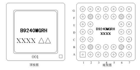
Figure 4-1. B9240MGRH pin description B9240MGRH pin description table
