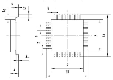
Figure 7-1 CQFP44 package specifications
