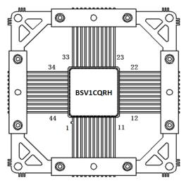
Figure 3-1 CQFP44 pin configuration
