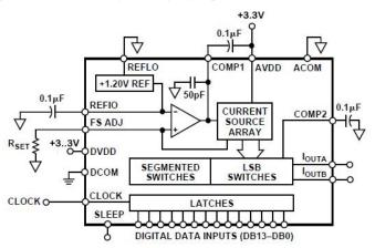
Figure 6 D/A Conversion Unit Functionnal Block Diagram
