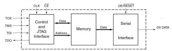
Figure 4 Configuration And Memory Unit Block Diagram
