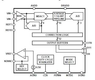
Figure 5 A/D Conversion Unit Functional Block Diagram
