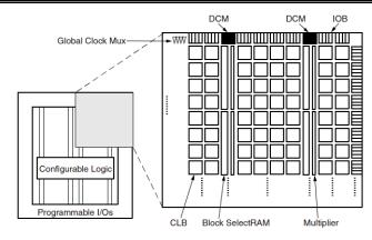
Figure 3 Programmable Logic Unit Architecture Overview
